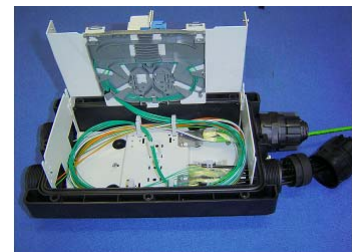
WTC1.5 with a splitter splice tray and SC adaptors on the top of the organizer
